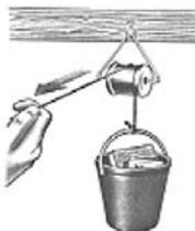
2. Bend about 8 inches of wire into a triangle shape and push the ends into a thread spool.
