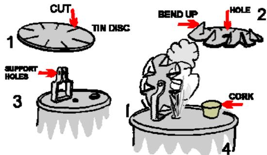
A Webelos Scout may get a graphic demonstration of the power of steam by building the simple steam turbine shown in this illustration. Materials needed are a tin can, a lid from a second tin can, a pair of tin snips, a sheet metal screw, a cork, a power drill, an extra piece of tin to make the support for the turbine wheel, a finishing nail, and a source of heat.
