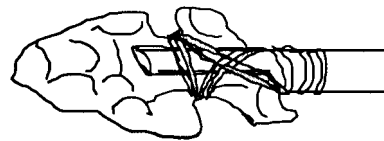
Apply epoxy and wrap sinew around arrowhead and shaft
