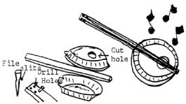
For the neck, place a strip of wood, about 2" wide, between the two pans (rims together). Attach tabs to the wood strips by hammering in tacks. At bottom of wood strip, hammer tacks in only half way for stringing wire.
